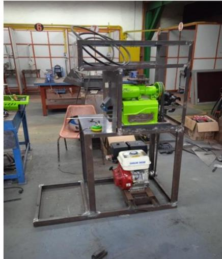
Gambar 2. Rangka Mesin Huller/Rice Milling
